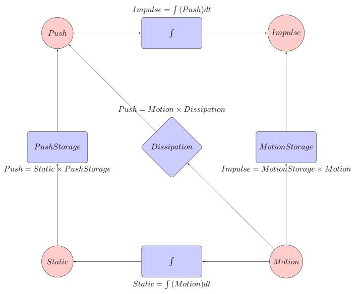
$$PushStoredEnergy = \frac{1}{2}PushStorage \times Static^2 = \frac{1}{2}\frac{Push^2}{PushStorage}$$
